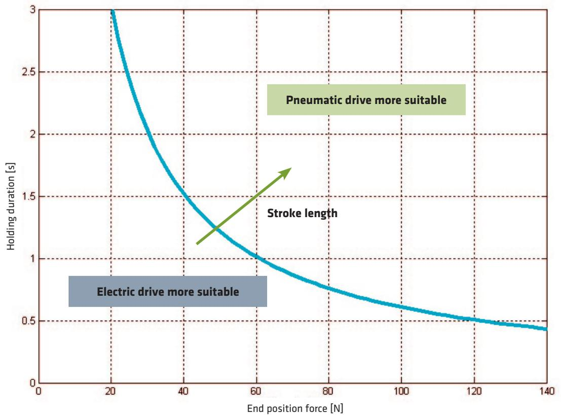
**Application-specific efficiency ranges for the holding handling function in both technologies.**
