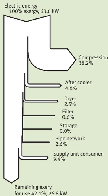
The figure on the left shows an example of an exergy flow diagram for a pneumatic system. Most of the exergy is lost on compression – 38.2% in the example shown here. At the end of the functional chain, an effective remaining exergy of 42.1% from the initial exergy is available for the application.
