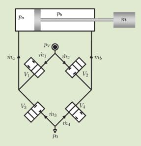
The individual valves are controlled based on optimisation. Using a mathematical system model in conjunction with numerical optimisation models enables an energy-efficient control with simultaneous reduction of the end position speed. The maximum permitted speed on impact in the end position can be taken into consideration in the optimisation algorithm. That eliminates the need to absorb the excess energy in the end position via
