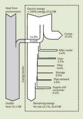
When the air is compressed, a lot of the heat development occurs in the compressed air chain due to thermodynamic effects. An essential factor for the efficiency increase of compressed air systems is therefore the integration of a heat recovery system. The heat can then be used for indoor heating or e.g. as process heat.
